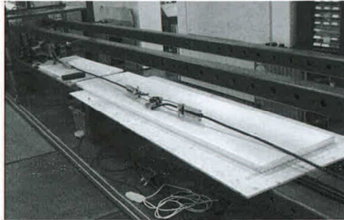
Picture 4: Test setup in tensile test machine (with out cooling device)
