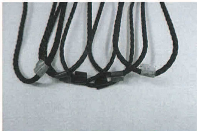
Picture 3: Identification markings washed after the test
