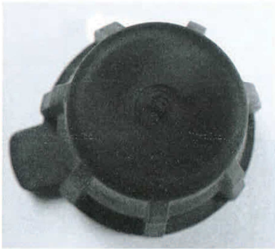
Picture 2: End cap before UV-test.
