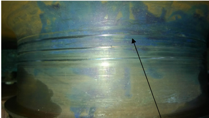
Oil labyrinth marks at coupling
